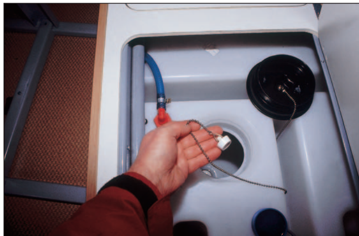
The inboard-mounted fresh water tank has a simple plug-on-chain draining system and a large inspection hatch for cleaning.
