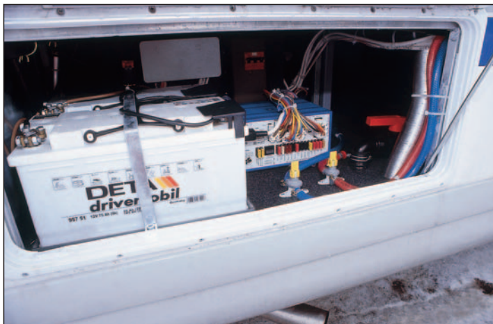
Open a nearside hatch and you have access to most of the service controls. Even the waste tank drain valve lives here in a back-friendly, muck-free environment.
