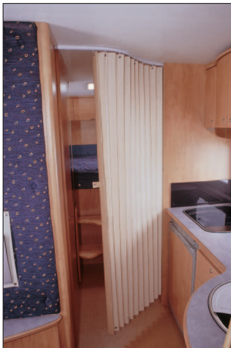
A room divider emerges from its slot to create en-suite facilities for the rear double.
